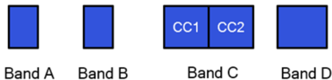
Figure 12: Switching band combination with more than 2 bands
