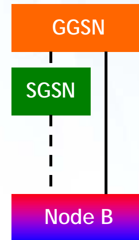
Possible HSPA+ with One-Tunnel Architecture
