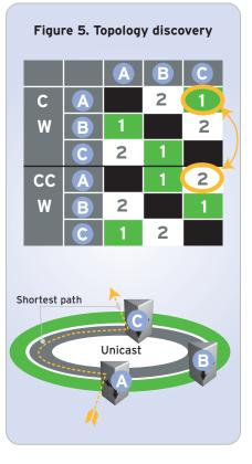
the ring during normal operation, which offer diverse routes in the event of a failure. There are two specific protection mechanisms specified for RPR as identified in Figure 4 — wrapping and steering.
