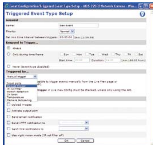
Figure 1.1.h. Setting up an event trigger using the network camera's user interface.
