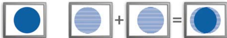
Figure 2.1.l. Freeze frame on moving dot using progressive scan
