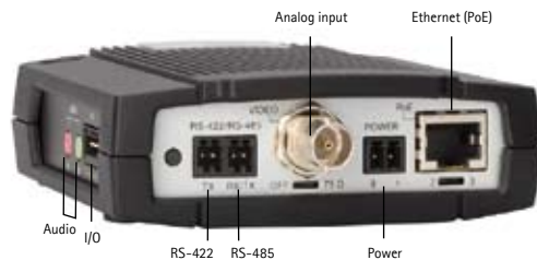
Figure 2.2.b. A one-channel, standalone video encoder with audio, I/O (input/output) ports for controlling external devices such as sensors and alarms, serial ports (RS-422/485) for controlling PTZ analog cameras and Ethernet connection with Power over Ethernet support.
