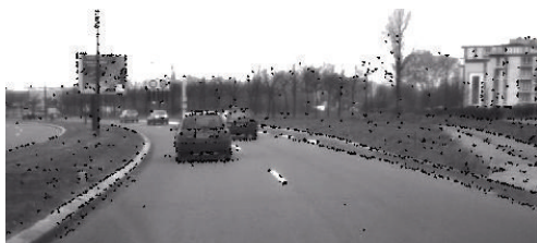
FIGURE 14.9. Real-time processing on a highway. The flies (black dots) concentrate on contrasted road edges and other cars.
