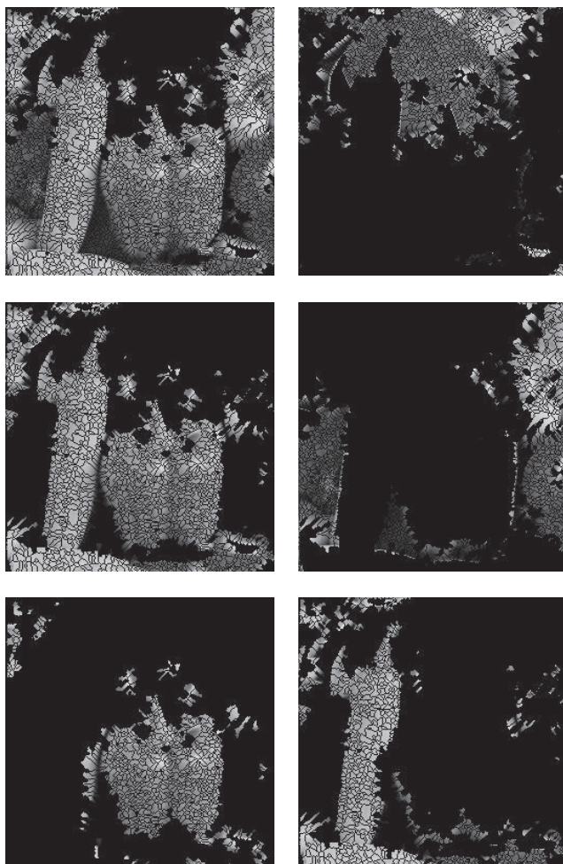
FIGURE 13.5. Application of the proposed method to the peppers image shown in Figure 13.4. The oversegmented image is bipartitioned in a hierarchical fashion. From top to bottom rows: First, second and third cut images. Left image in each row is hierarchically subdivided.
