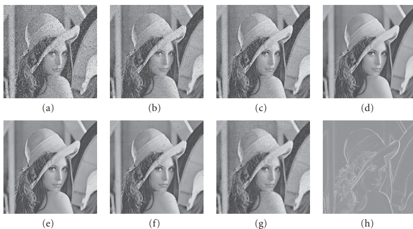
FIGURE 5.10. Corrupted and filtered images: salt and pepper noise ((a) versus (e)), random shot noise ((b) versus (f)), Gaussian noise ((c) versus (g)), edge detector ((d) versus (h)).
