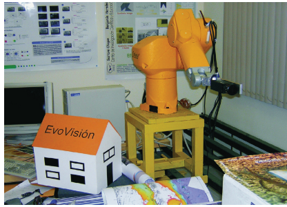
FIGURE 19.1. Typical sensor planning research is carried out with a robot manipulator and a CCD camera in what is known as a hand-eye configuration.
