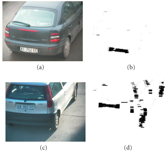
FIGURE 3.7. Typical results: the case reported above is quasi-ideal. In cases like the one reported below, despite the very “noisy” output, the distribution of the false detections is such that the license-plate region can be easily detected anyway.
