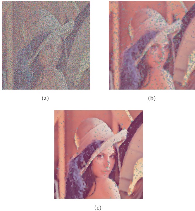
FIGURE 11.10. Filtering in the presence of large amounts of impulse noise. (a) Lena image with 70% random impulse noise. (b) Effect of vector median filtering. (c) Effect of vector mode filtering. Both of the filters are applied in a 9 \times 9 window. (Reproduced from D. Charles and E. R. Davies, "Mode filters and their effectiveness for processing color images," Imaging Science Journal © 2004 RPS.)
