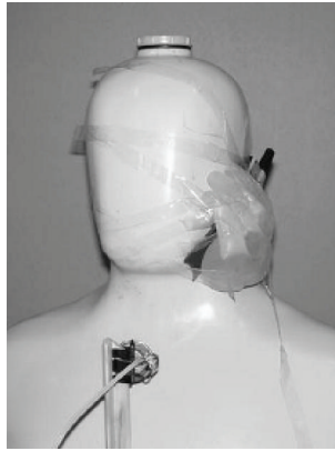
FIGURE 2.29. Human torso phantom used for radiation measurements in the GSM and UMTS frequency bands [164].
