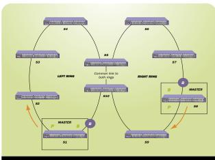
Figure 5: VLANs in Multiple EAPS
