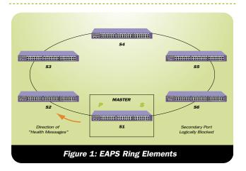
An EAPS domain is configured to protect a group of data carrying virtual local area networks (VLANs), called protected VLANs as shown is Figure 2. There could be multiple EAPS domains running on the same switch, each with its unique control VLAN. Similarly, many domains can co-exist on the same ring protecting different sets of VLANs.
