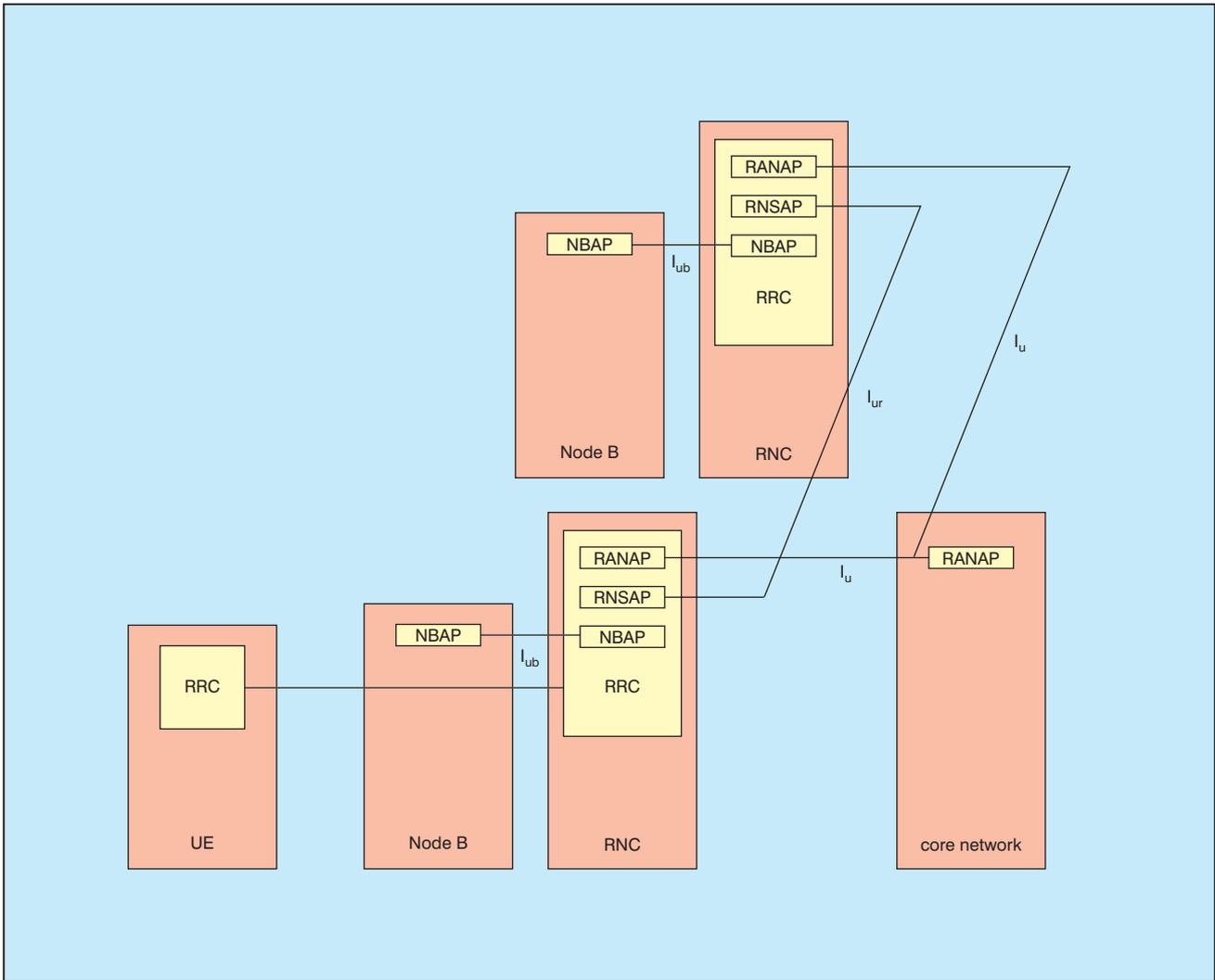
Fig. 7 Radio resource control signalling protocols
