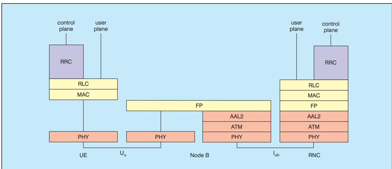
Fig. 6 Simplified protocol diagram
