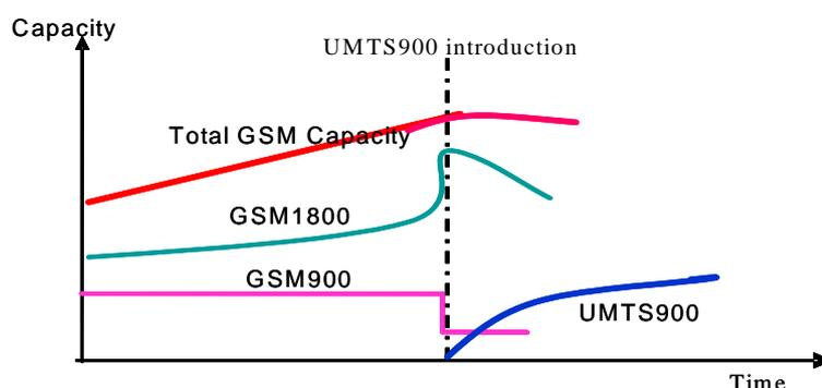
Figure 7: Load balancing between GSM900 and GSM1800 in a dualband GSM network in order to refarm part of GSM900 spectrum for UMTS900 deployment
