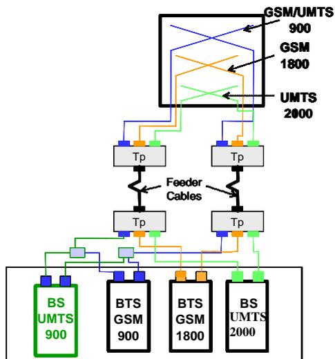
Figure 6: Radio site design example for GSM-UMTS900/GSM1800/UMTS2000 with a tri-band polarization diversity antenna (Tp=Triplexer)
