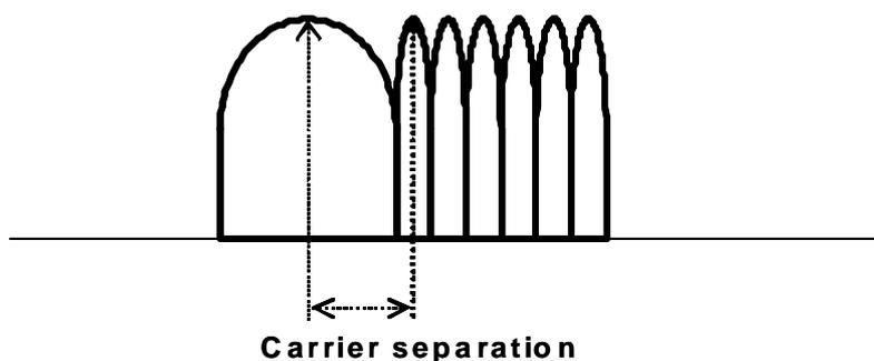
Figure 3 – Carrier separation between UMTS900 and GSM900
