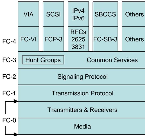
Figure 1 Fibre Channel Structure
