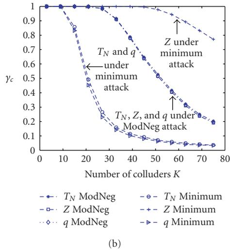
FIGURE 3.13. (a)  $P_d$  and (b)  $\gamma_c$  of different statistics under the minimum attack and modified negative attack with bounded Gaussian-like fingerprints. Here  $\sigma_W^2 = 1/9$ ,  $M = 100$ , and  $N = 10^4$ .  $P_{fp} = 10^{-2}$  in (a) and  $\gamma_i = 10^{-2}$  in (b).
