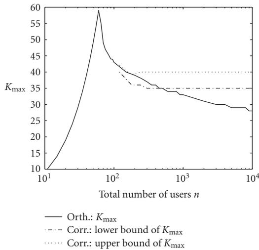
FIGURE 5.3. Comparison of collision resistance of the orthogonal and the proposed group-based fingerprinting systems to the average attack. Here  $M = 60$ ,  $k_i = K/|i|$ ,  $|i| = 5$ , and the system requirements are represented by  $\epsilon = 10^{-3}$  and  $\beta = 0.8$ .
