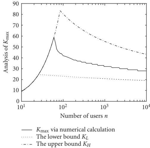
FIGURE 4.4. The lower and upper bounds of  $K_{\max}$  as a function of the number of users  $n$  when applying the thresholding detector in (4.9). Here  $WNR = 0$  dB,  $N = 10^4$ ,  $\epsilon = 10^{-3}$ , and  $\beta = 0.8$ .
