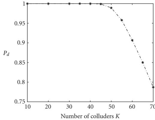
FIGURE 4.10. The detection performance of the thresholding detector on Lena images under the average attack, where equivalently  $N = 13\,691$ . Here  $\sigma_a^2 = 1$ ,  $n = 100$ , and  $P_{fp} = 10^{-3}$ .
