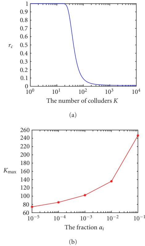
FIGURE 4.5. The resistance performance under the criteria  $r_c$  and  $r_i$ , when applying the thresholding detector in (4.9). (a) We plot the expected fraction  $r_c$  versus the number of colluders  $K$ , with  $N = 10^4$ , the WNR  $\eta = 1$ , and the expected fraction  $r_i = 0.01$ . (b)  $K_{\max}$  under different requirements of  $\alpha_i$  with  $N = 10^{-5}$ , the WNR  $\eta = 1$ , and  $d_c = 0.5$ .
