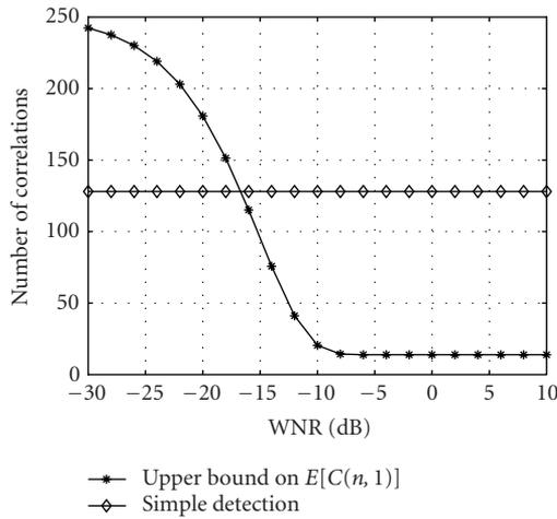
FIGURE 4.13. The bound for the expected amount of correlations needed when there is one colluder,  $n = 128$  users, and  $P_D = 0.99$  for each level. As a baseline, we plot the bound for  $E[C(128, 1)]$  against the amount  $n$ , which is the amount of computations needed in performing simple detection.
