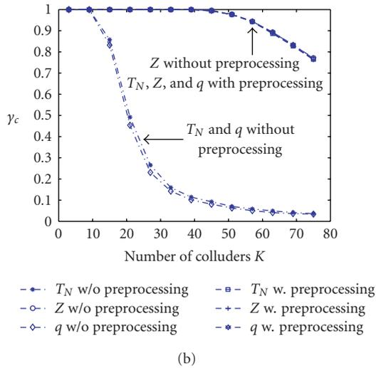
FIGURE 3.15. Performance of the detection statistics under the minimum attack with and without preprocessing. Fingerprints are generated from bounded Gaussian-like distribution (3.61) with  $\sigma_W^2 = 1/9$ ,  $M = 100$ , and  $N = 10^4$ . In (a),  $P_{fp} = 10^{-2}$  and we compare  $P_d$  with and without preprocessing. In (b),  $\gamma_i = 10^{-2}$  and we plot  $\gamma_c$  with and without preprocessing.
