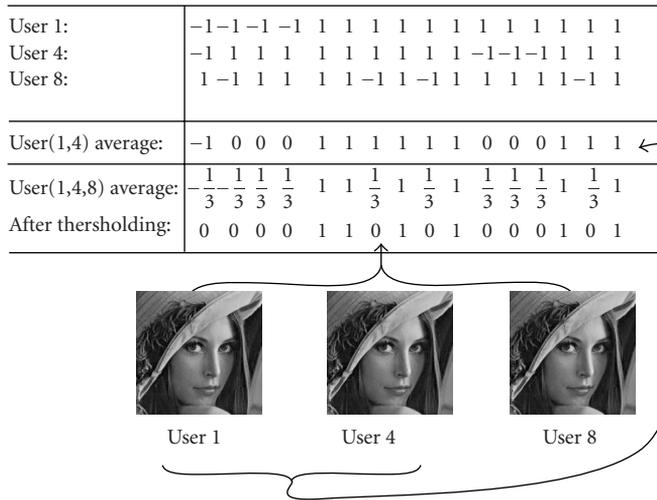
FIGURE 6.3. 16-bit codevectors from a (16, 4, 1)-ACC code for users 1, 4, and 8, and the fingerprinted 512×512 Lena images for these three users, respectively. The code can capture up to 3 colluders. Shown here is an example of two-user collusion by averaging (users 1 and 4) and an example of three-user collusion by averaging. The two codes indicated by arrows in the table uniquely identify the participating colluders.
