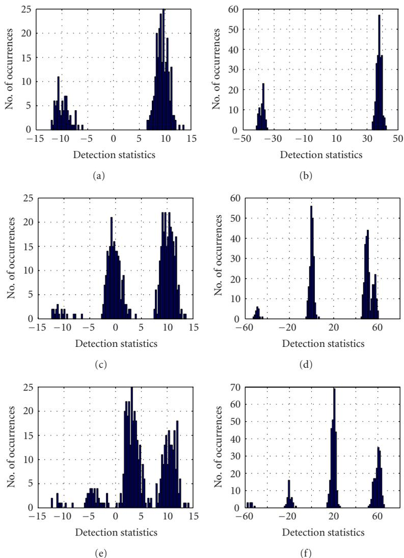
FIGURE 6.10. Histograms of detection statistics  $\{T_N(i)\}$  of embedded fingerprints: (top row) single-fingerprint case, (middle row) two-user collusion case involving users 1 and 4 as colluders, (bottom row) three-user collusion case involving users 1, 4, and 8 as colluders; (left column) blind detection, (right column) nonblind detection.
