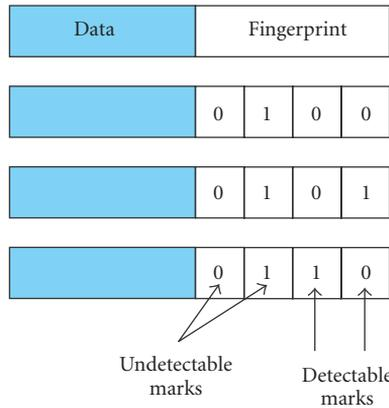
FIGURE 6.1. Illustration of the marking assumption.
