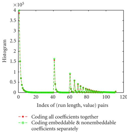
FIGURE 7.7. Histograms of the (run length, value) pairs of the “carphone” sequence that are variable-length coded in the two schemes.  $R = 1$  Mbps. The indices of the (run length, value) pairs are sorted first in the ascending order of the run length, and then in the ascending order of the value: (a) in the intracoded blocks; (b) in the intercoded blocks.
