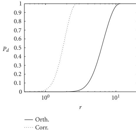
FIGURE 5.5. Performance curves  $P_d$  versus  $r$  of different examples, compared with the orthogonal scheme in [58]. In (a)  $K = 23$ , a small number of users  $n = 40$ , and a negative  $\rho = -0.023$  are considered. In (b) a large number of users  $n = 600$  and a positive  $\rho = 0.3$  are considered. Three groups are involved in collusion, with numbers of colluders being 32, 8, and 8, respectively.
