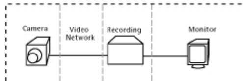
**Digitization of the Camera.** Digitization in the CCTV arena began around 1990 when digital cameras (based on CCD sensors) replaced analog tube cameras. These CCD cameras were *partly* digital, but they still used analog connections of coax cable for the composite video, and recording was still done to analog VCR tapes. We'll refer to this technology period as the **VCR era**.
